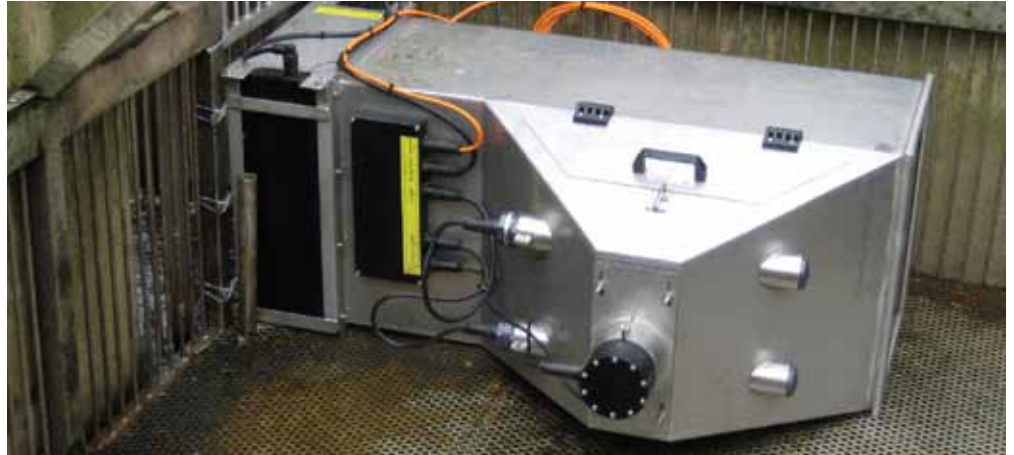
The camera, lights and scanner are connected to the PC through the connection box.
